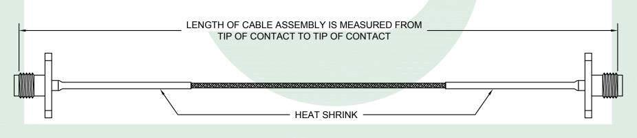
SMA FEMALE 2 HOLE PANEL MOUNT CONNECTOR A
